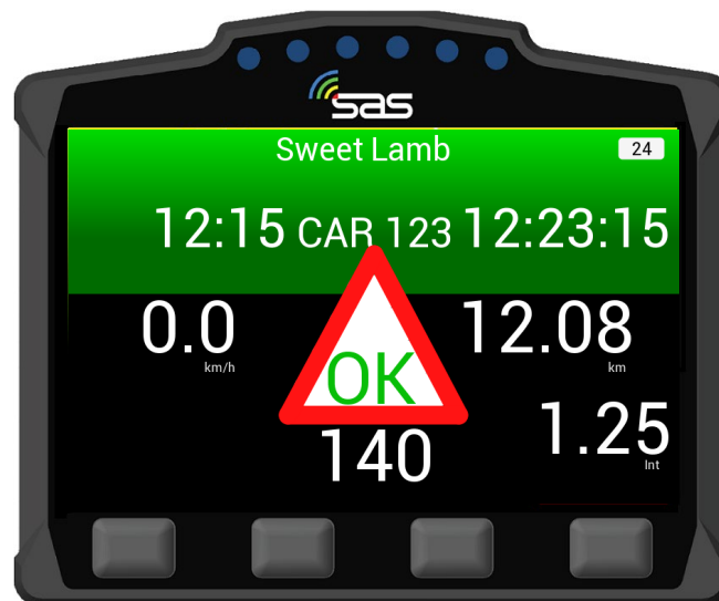
SCREEN 10. OK proximity warning
