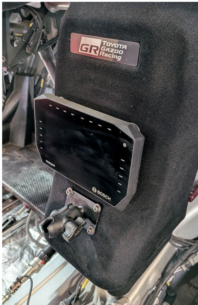
Figure 3. 25mm rubber ball securely attached to the dashboard
